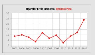
For operator error incidents that occur within facilities, the data does not show a similar, drastic increase since 2010. However, the data does indicate that the largest share of incidents¹ result from tank overfills/overflows. More than half of the tank overfills/overflows involve sumps/separators. Given this fact, pipeline operators consider installing overflow indication on sumps/separators and reviewing procedures for responding to indications from these devices.
