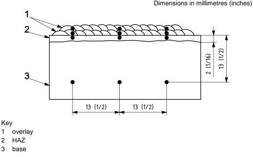
Figure 6 — Hardness test locations for weld overlays
